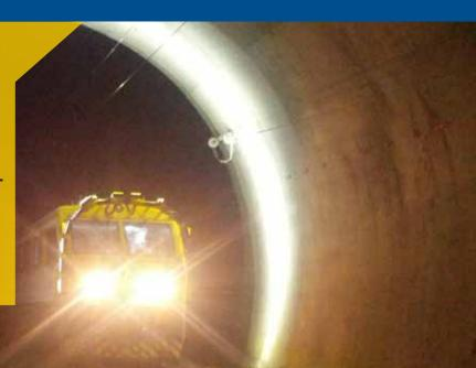
**Tunnel Scan System (TS)** uses multiple high-speed linear cameras and laser scanner to acquire 2D images and high resolution 3D profiles of tunnel wall.
